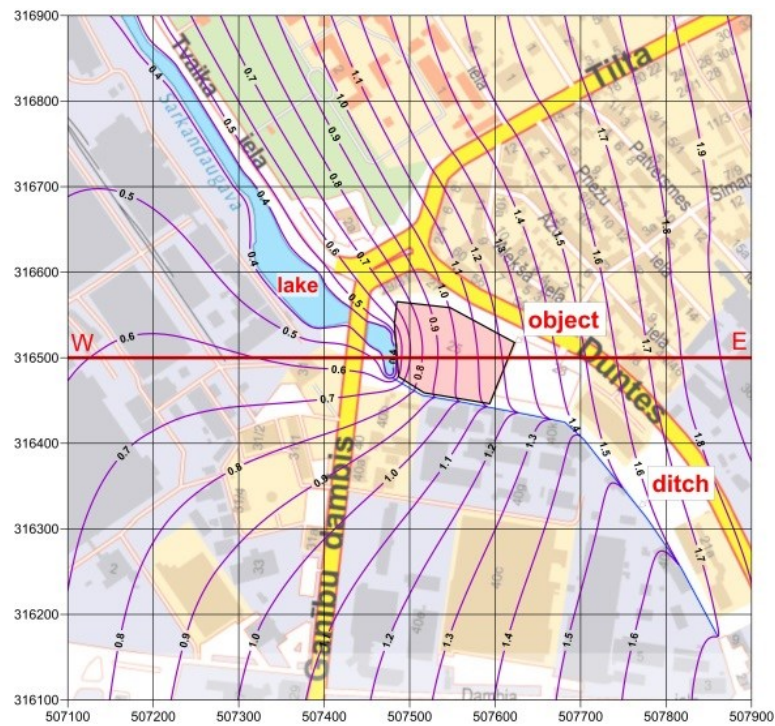
Fig. 2. The groundwater head isolines [m asl] of the layer Q27. The cross section W-E location is shown
